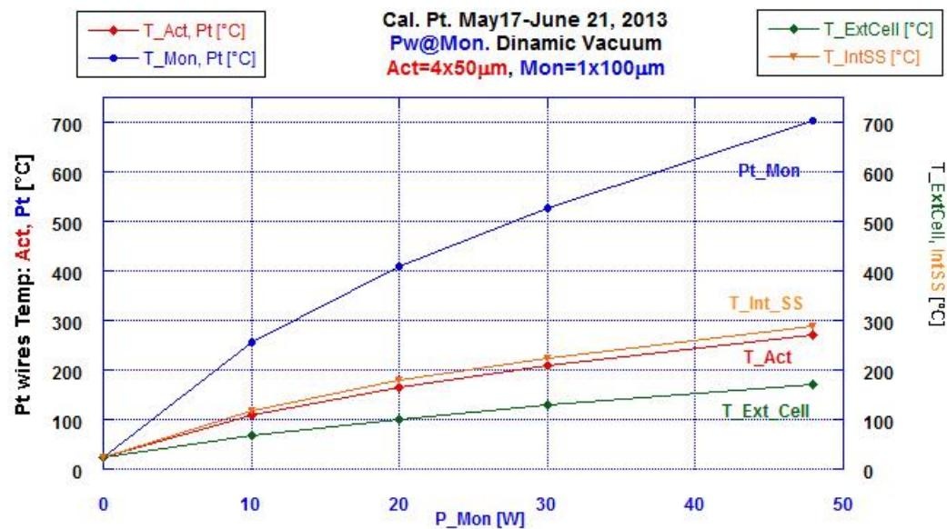
**Pt wire, Pw applied to Mon wire. Measurement of mean Pt wire temperature by resistive thermal coefficient values. Cross-ceck by visual observation, color, at higher powers: starts red color almost uniform.**
