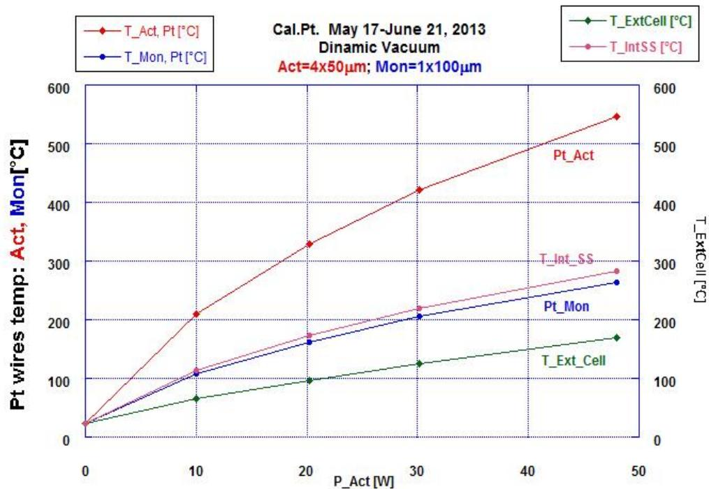
**Pt wire, Pw applied to Act wire. Measurement of mean Pt wire temperature by resistive thermal coefficient values. Cross-ceck by visual observation, color, at higher powers: only limited wire sections start light-red colors.**
