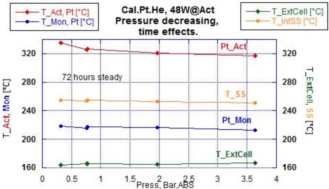
Pw at Pt\_Act., 48W. He atmosphere. Effect of pressure variation on Pt\_Act and Pt\_Mon. temperatures: they increase as the pressure decreases. Also The internal cell temperature (T\_SS) increases. **Only the External Cell (ExtCell) temperature (green color) decreases.**
