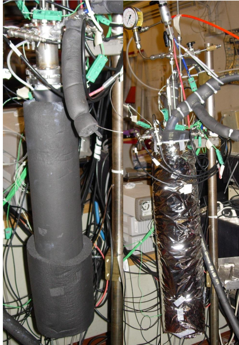
Real reactor: steps 6-7 of assembly, final thermal insulation.
